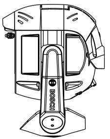
Figure 10.1: Sunshield installation is complete.
