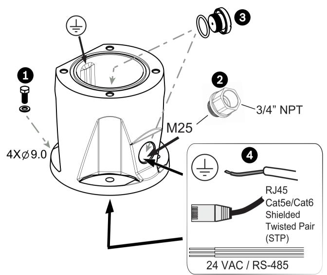
1. Attach the DCA to the mounting location using user-supplied hardware (item 1). (Bosch recommends stainless steel bolts and washers.)
