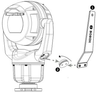
Figure 12.2: Remove the yoke caps with the spanner tool.
