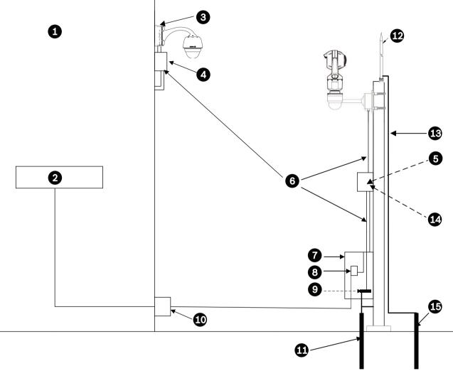
Figure 19.1: Correct outdoor installation with proper surge/lightning protection
