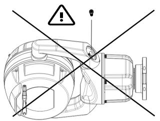
Figure 12.1: Do NOT allow screws or other objects to fall inside the camera.
