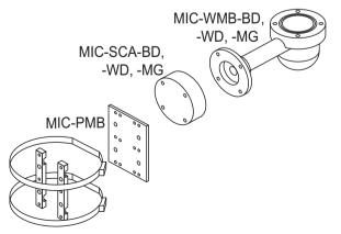
Figure 5.3: Typical Pole mount configuration
