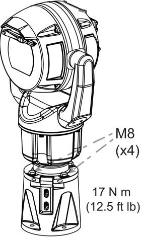
12. Carefully tip the camera to its final position. Avoid pinching wires between the camera base and the DCA! Insert four washers and hex bolts (supplied).
