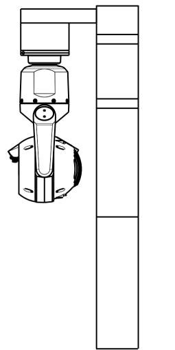
Figure 5.6: MIC camera mounted in inverted orientation (on pole)
