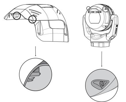
5. Install the M4 x 10 screws. Tighten the screws to 2.2 N m (19.5 in-lb).
