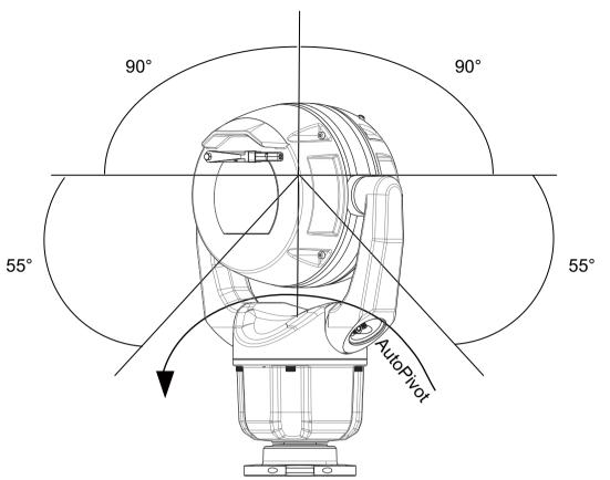
Figure 5.1: Tilt range, MIC IP ultra 7100i
