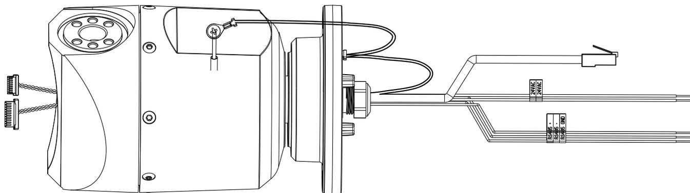
11. Connect the lead from the camera pigtail to the ground post on the pan base. The connection for the customer should be to the lead from the post.
