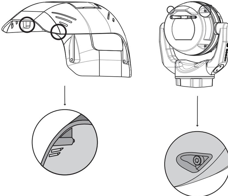
5. Install the M4 x 10 screws. Tighten the screws to 2.2 N m (19.5 in-lb).
