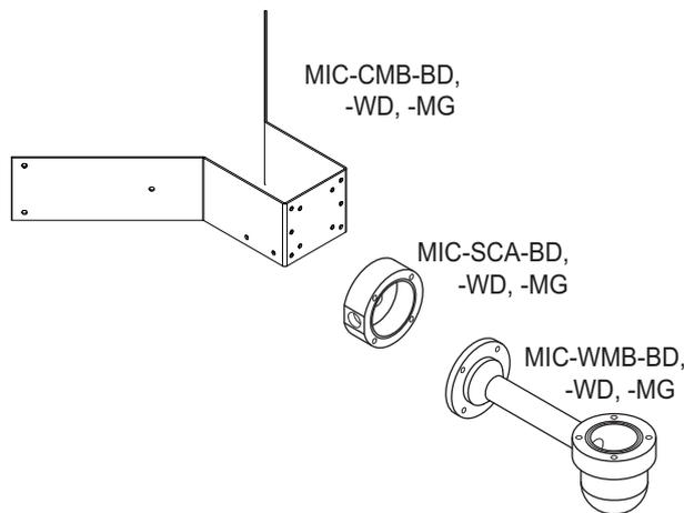
**Figure 5.4: Typical Corner mount configuration**
