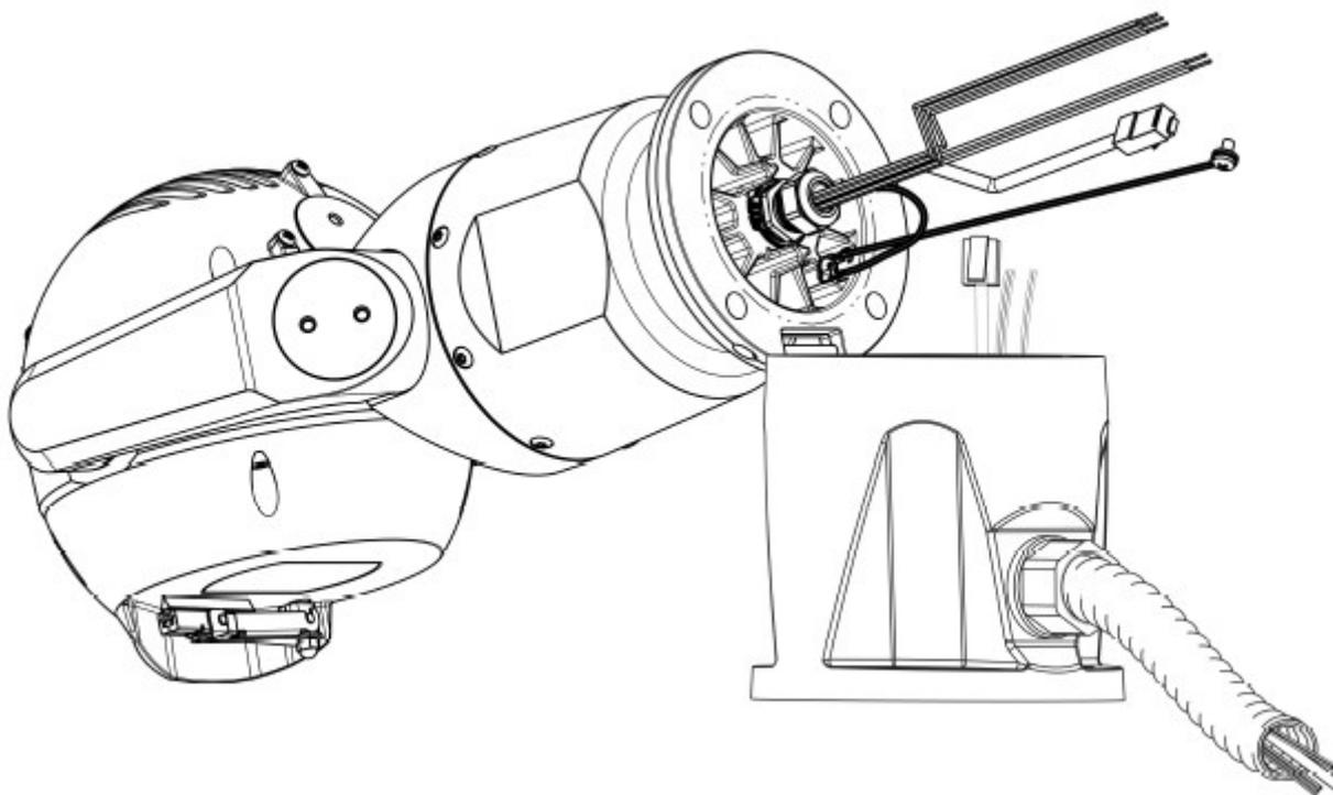
9. Carefully tilt the camera to the side with the pin under the hook.
