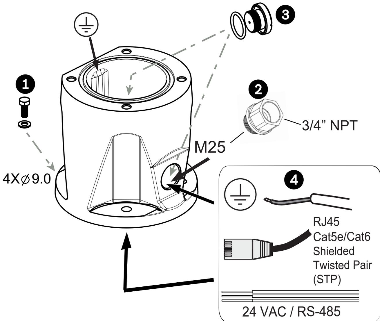
1. Attach the DCA to the mounting location using user-supplied hardware (item 1). (Bosch recommends stainless steel bolts and washers.)
