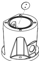
Bosch suggests storing the access plug inside the DCA mount (or wall mount accessory) in case it becomes necessary to remove the illuminator.
