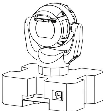
4. Supply power to the camera and *Connect the Camera to the Network*, page 43. Note that the wiper moves one to three times across the camera window, and then returns to parked position.
