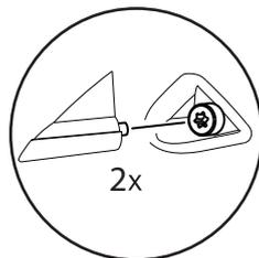
4. Make sure that the tabs in the sunshield lock into place in the camera head.
