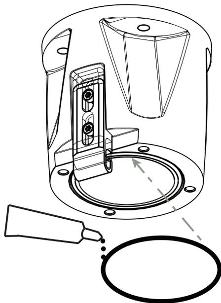
7. For inverted installation, apply a small amount of grease to the primary O-ring to hold it in place.
