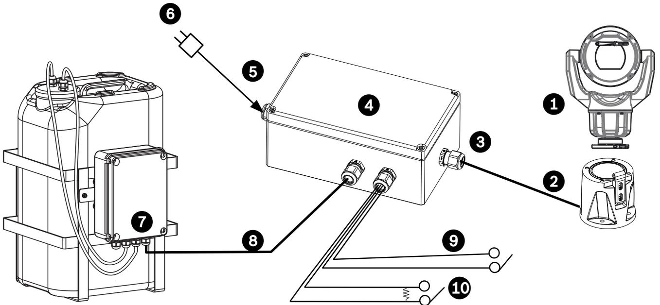
Figure 14.2: System Configuration with an MIC Alarm-Washer Box (MIC-ALM-WAS-24)
