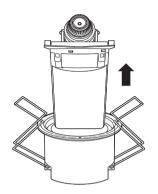
4 Use a 83-86mm(3.25"-3.4") diameter hole saw
