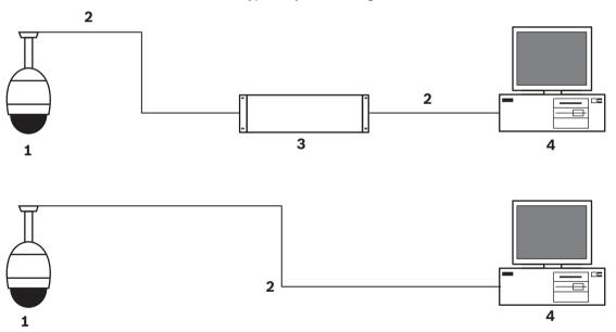
Figure 11.1: AUTODOME IP System Config
