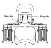
4. Connect the power cable and RS-485 cable of the IR illuminator to the board in the housing.
