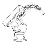
Connect the IR illuminator to the fixed bracket, using 3 bolts as shown.
